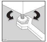
Any necessary adjustment can be made with a spanner. Accurate levelling prevents vibration, noise and displacement of the machine during operation. Some vibration is inevitable, especially if mounted on a wooden floor. Sprung wooden floors are particularly susceptible to vibration. For advice, consult a builder. If possible, always place the machine on a solid floor.
